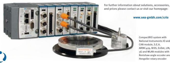
CompactRIO system with National Instruments IO and CAN module, S.E.A. ARINC429, BiSS, EnDat, LIN, 3G and WLAN modules with Renishaw angle eccoder and Hengstler rotary encoder
